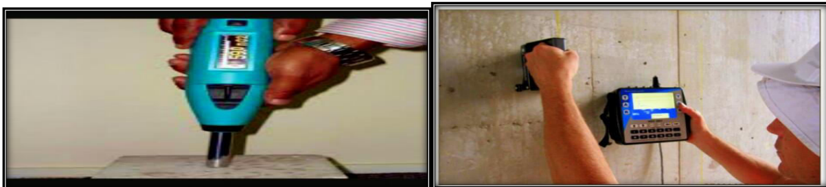
Fig 2 (a) Rebound Hammer Test. Fig 2 (b) Impact Echo Test.
