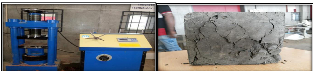
Fig 1 (a) Compressive Testing Machine. Fig (b) Sample Cube
